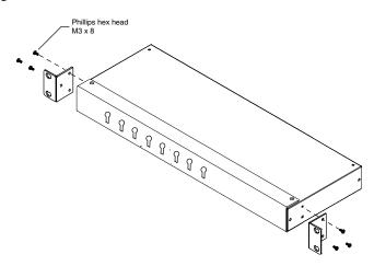
3. Slide the unit into the rack and secure it to the rack.
